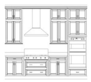
A floor-level drawing that shows a front, side or rear view of a room in a vertical plane, illustrating how elements appear face-to-face in the space.
