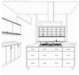
A perspective drawing is one that is "3D" or dimensional. It shows the room as it would be actually seen from the viewpoint of a person 5'-6" in height. Perspective drawings provide details such as areas that are increased or reduced in depth, a dimensional quality that elevation drawings don't offer.
